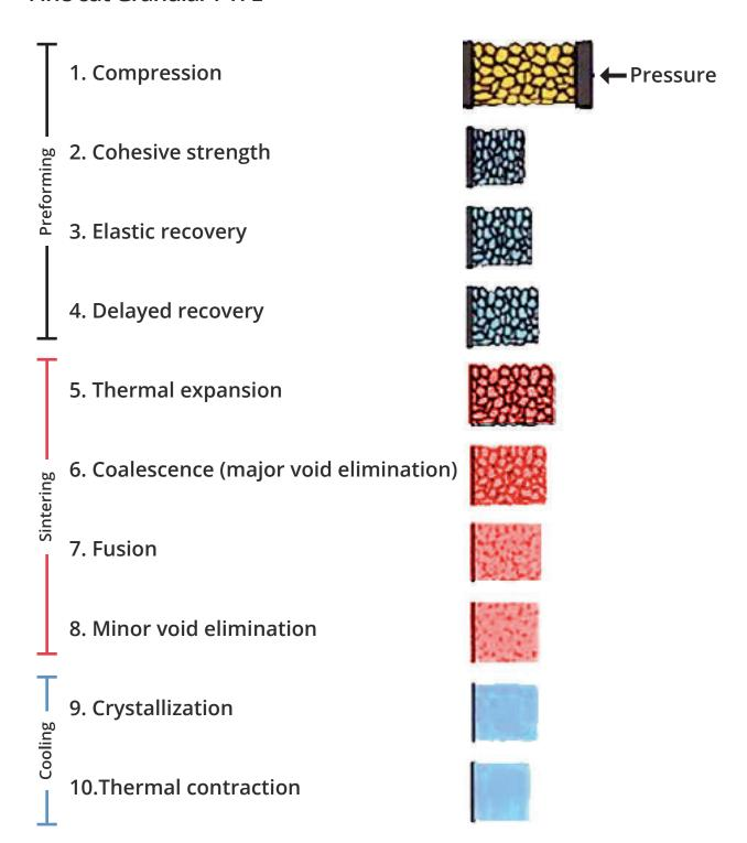
Figure 1- Schematic diagram of preforming and sintering sequence with PTFE
